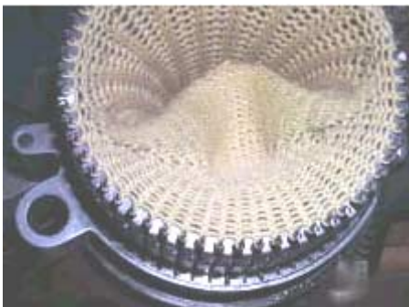
Note heel pouch inside cylinder
